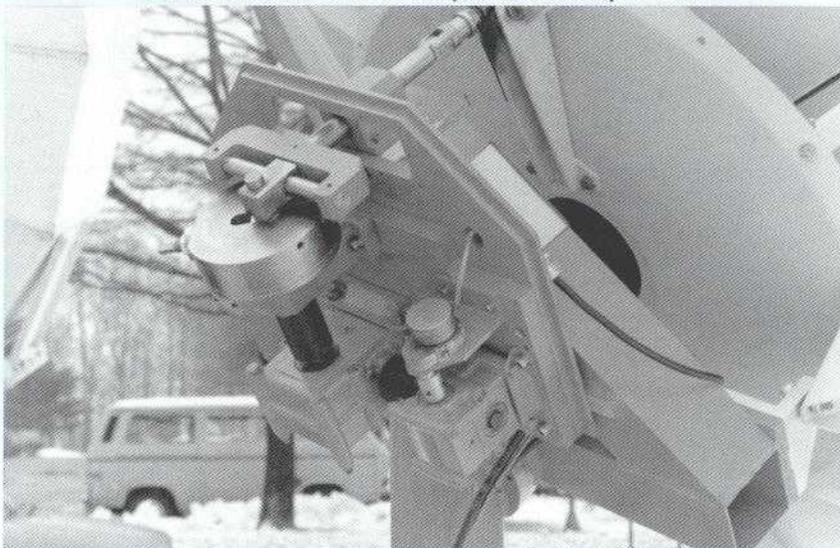
COMSAT General has developed a tracking antenna mount for use with "COMSAT Maneuver" satellites operating in inclined orbits. The mount is intended for use with small aperture antennas and is suitable for C or Ku band operation.
