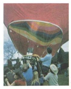
velope at the bottom and nearest the burners-is easily scorched. The crew must work quickly to keep the fabric away from the flame.
