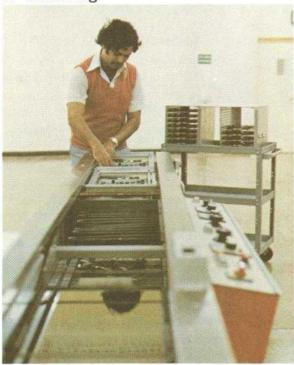
George Oomman operates the drag solder machine, which applies solder to PC boards.
