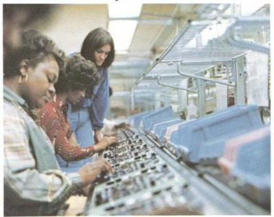
What automatic insertion machine can't do is done by hand in a slide-line operation. (Employee adds some components, then slides board to next person.) Left to right: Martha Ward, Barbara Floyd and Diane Allen, Supervisor, Manufacturing.
