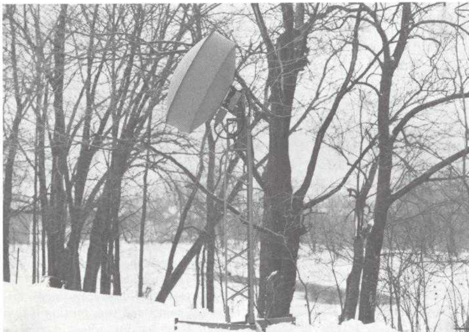
A small antenna transmits hydrological data by satellite to receive points in the United States and Canada.
