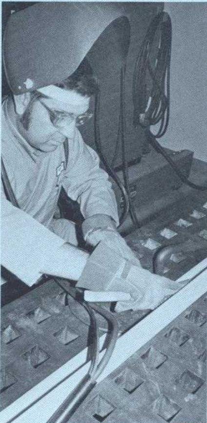
Al Eaton cleans a welded joint.
