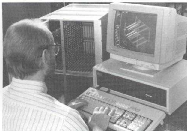
Figure 6. TDMA subrack chassis
