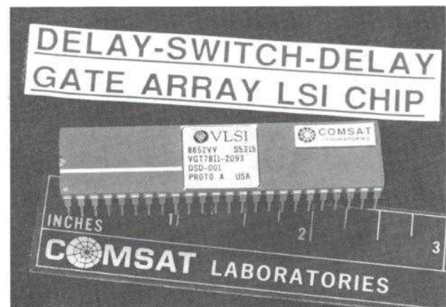
Figure 1. Delay/switch/delay ASIC chip
