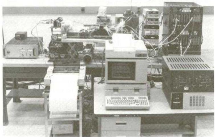
Figure 5. Equipment for multiple stress testing of TWTAs
